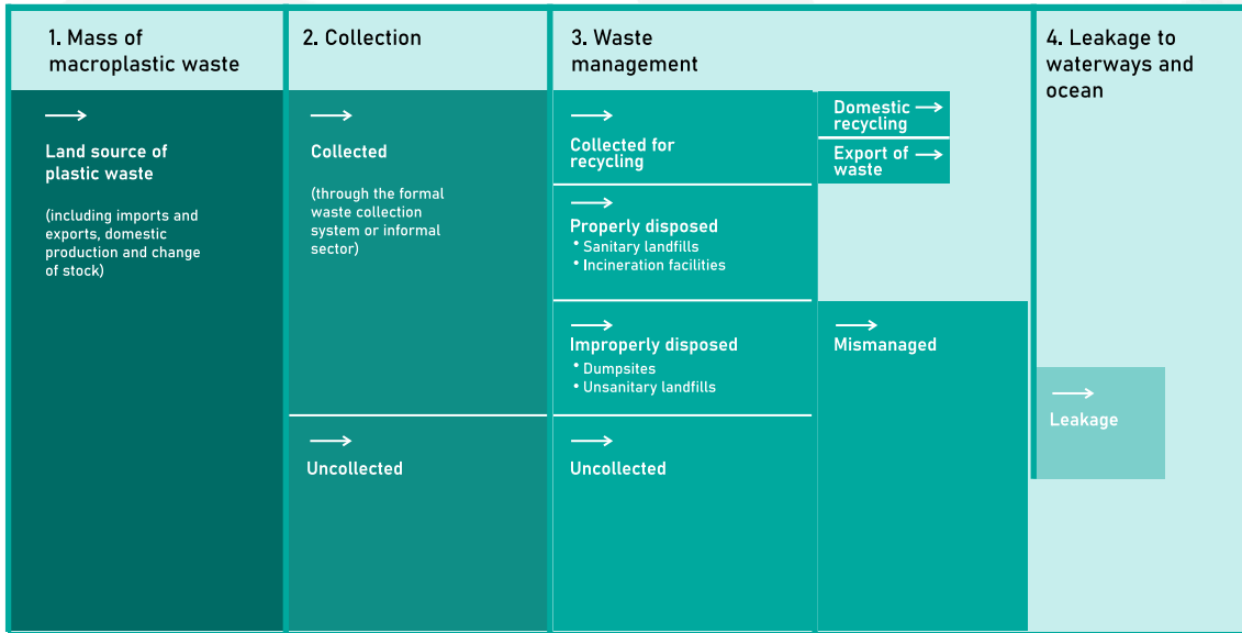
Figure 2-7: UNEP's definition of a Plastic Leakage Pathway
